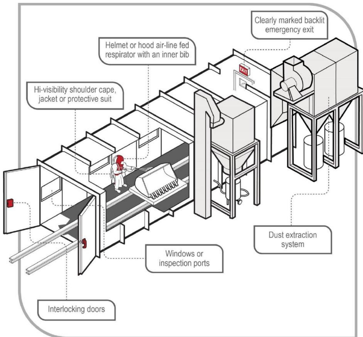
Figure 2 Blasting chambers
