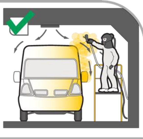
FIGURE 8 The use of a gantry or lift avoids overspray on to the operator, and avoids them having to stretch and reach
