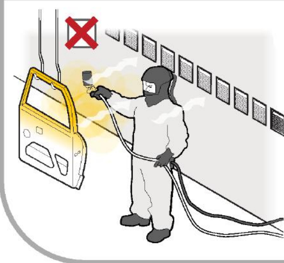
FIGURE 1 The operator is exposed to overspray because of poor positioning in relation to the airflow
