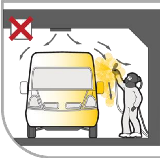
FIGURE 7 The operator is exposed to overspray and reaching above shoulder height can cause discomfort and injury to the body
